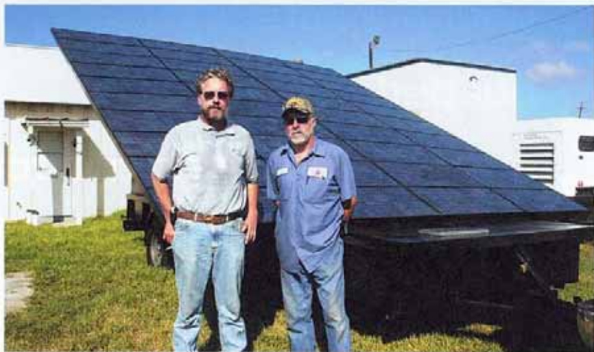
On line: Bill Ball (left) poses with port technician «Buddy» in front of his 2.4 kW mobile PV system, here powering equipment at a New Orleans port's temporary offices.
